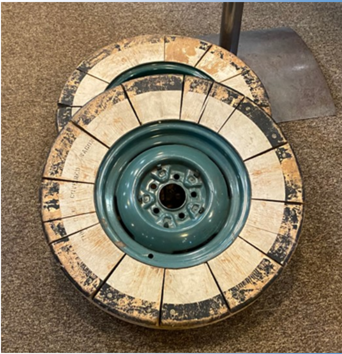
The original Jeep concept vehicle is to the left and above they experimented with wood wheels during the rubber shortage during WWII
