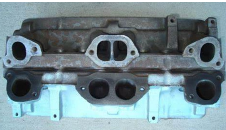
Side by side comparison of the Ram Air III (D port head on top) and the Ram Air IV (Round port head on bottom)
