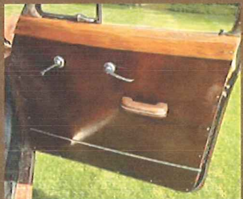
Pontiac station wagons in 1950 featured all-metal exteriors, yet a few wooden interior trim pieces remained including door panels such as the example shown here.
